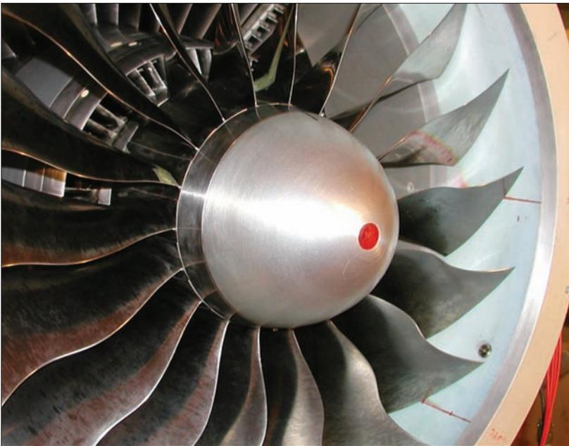
*A 22-in. scale model of a NASA/Pratt & Whitney geared turbofan was tested in the NASA 9x15-ft Acoustic Wind Tunnel.*
