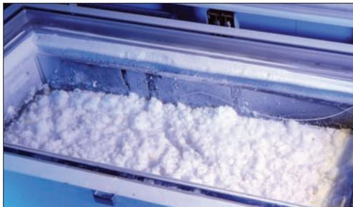
*A frozen basic hydrogen peroxide batch is used to demonstrate long-term fuel storage for chemical oxygen-iodine laser operation at the German Aerospace Center (DLR) Institute of Technical Physics. Photo courtesy DLR Institute of Technical Physics.*
