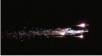
The Hayabusa capsule, which returned to Earth after a seven-year journey to asteroid Itokawa, is seen on the right, leading the debris and disintegration of the spacecraft. Courtesy JAXA/NASA.
