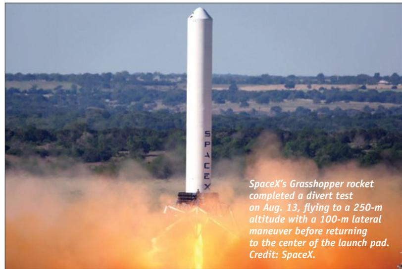
*SpaceX's Grasshopper rocket completed a divert test on Aug. 13, flying to a 250-m altitude with a 100-m lateral maneuver before returning to the center of the launch pad. Credit: SpaceX.*
